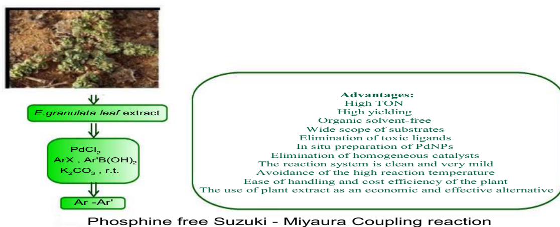
Scheme 18 Phosphine free Suzuki–Miyaura coupling reaction catalyzed by PdNPs [54]
